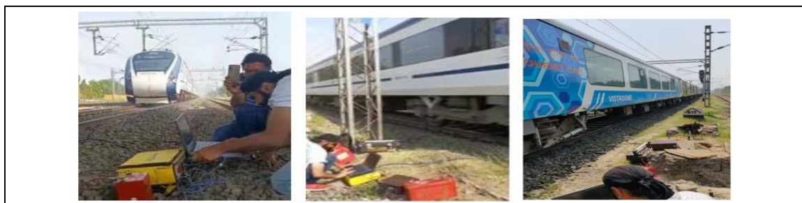
Figure. 3 SASW Test arrangement on Vande Bharat and Tejas Exp on progress
