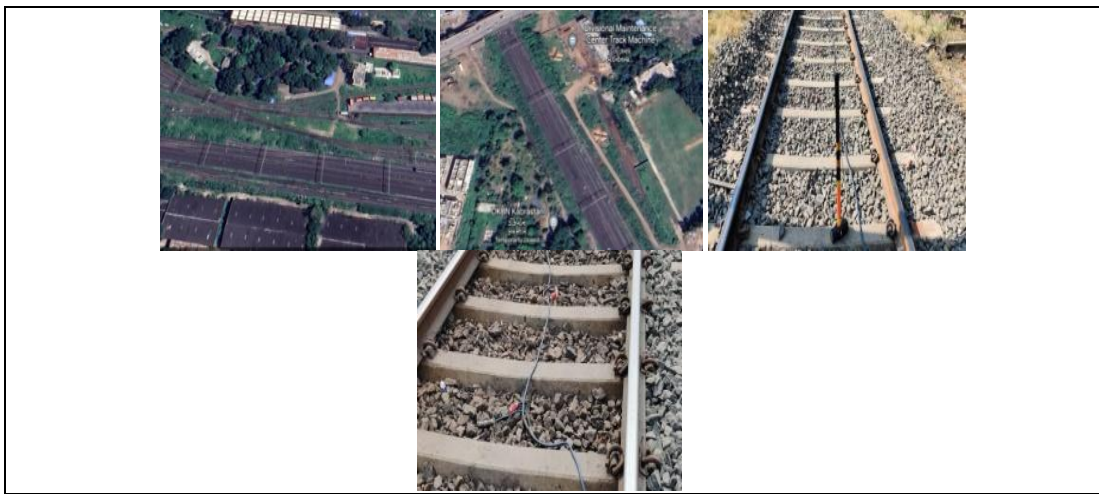
Figure 1: Location A & B, SASW Field setup for Local trigger mode, Geophone arrangement
