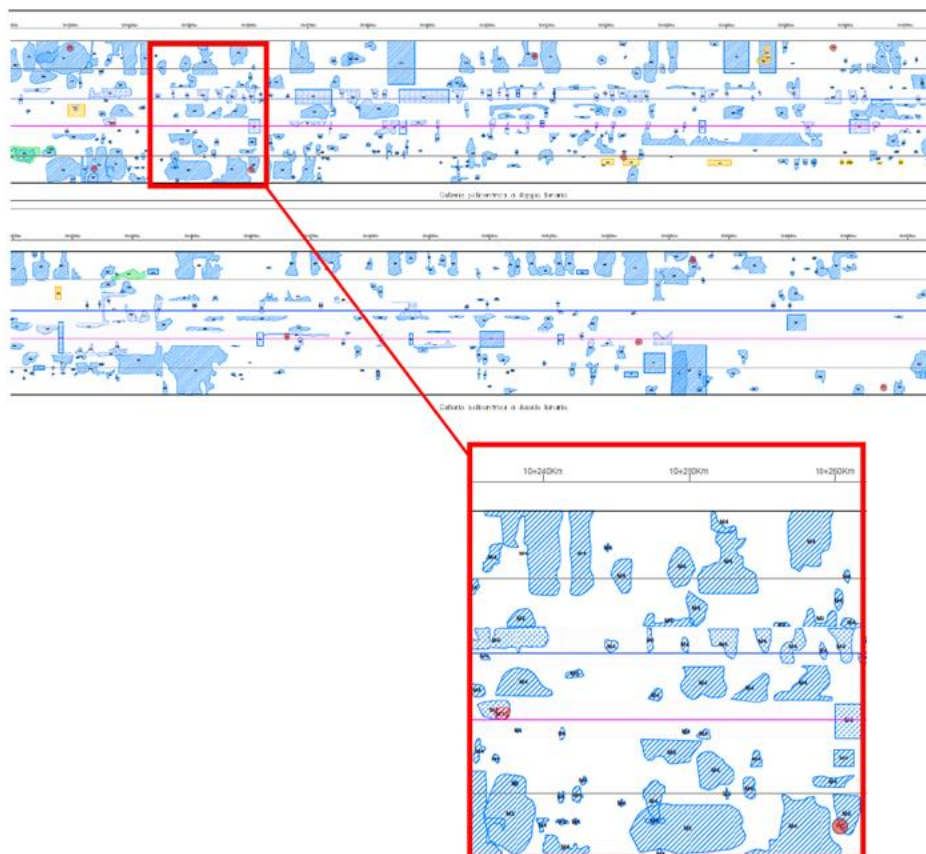
Figure 9: Example Defect Map.
