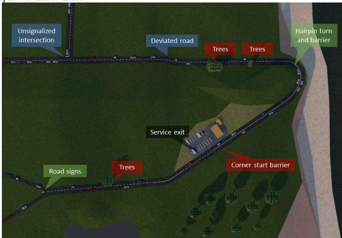
Figure 5: Test scenario with 8 different dangerous points.
