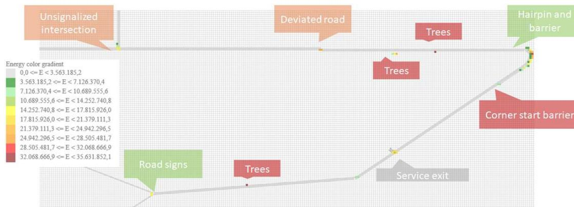
Figure 6: Six dangerous points can be easily spotted with high crash energy values.
