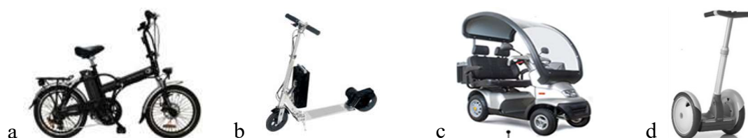
Figure 1: Examples of ATMs: (a) an e-bicycle; (b) an electric scooter; (c) a mobility scooter; (d) a segway.
