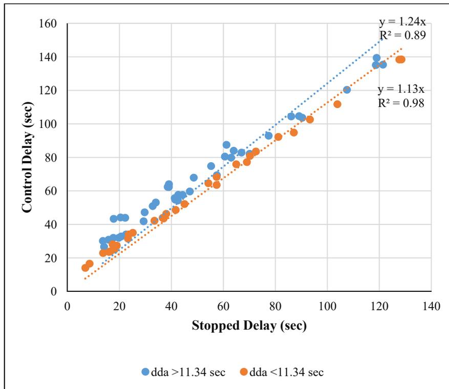
Figure 7: Relation between stopped delay and control delay for different deceleration-acceleration delay.
