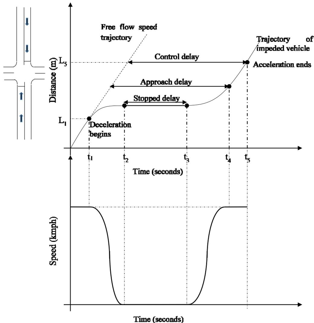
Figure 1: Distance-time and speed-time diagram of a stopped vehicle at the signalized intersection.
