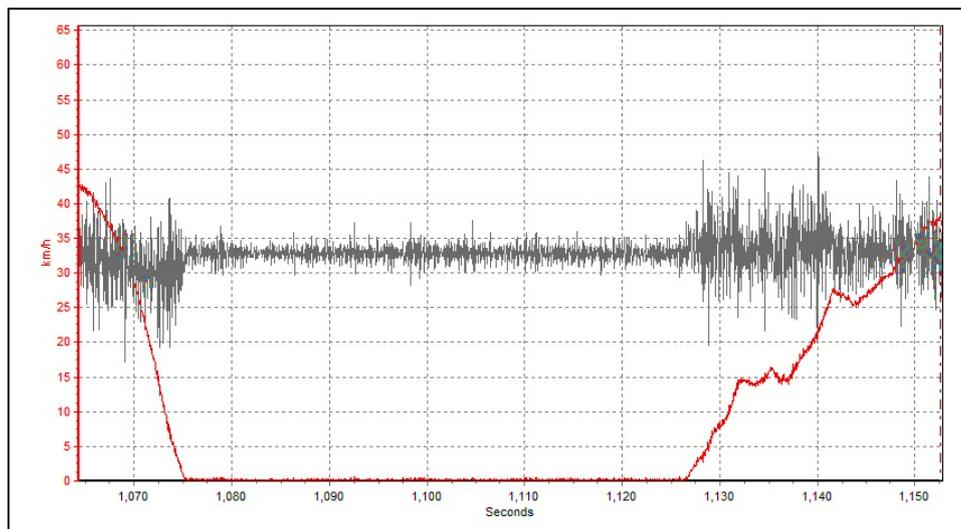
Figure 4: Speed and acceleration profile of a stopped vehicle at signalized intersection.
