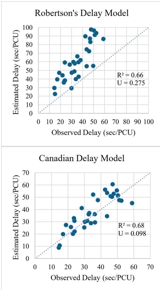
Figure 8: Relation between the field observed delay and the various delay model estimates.
