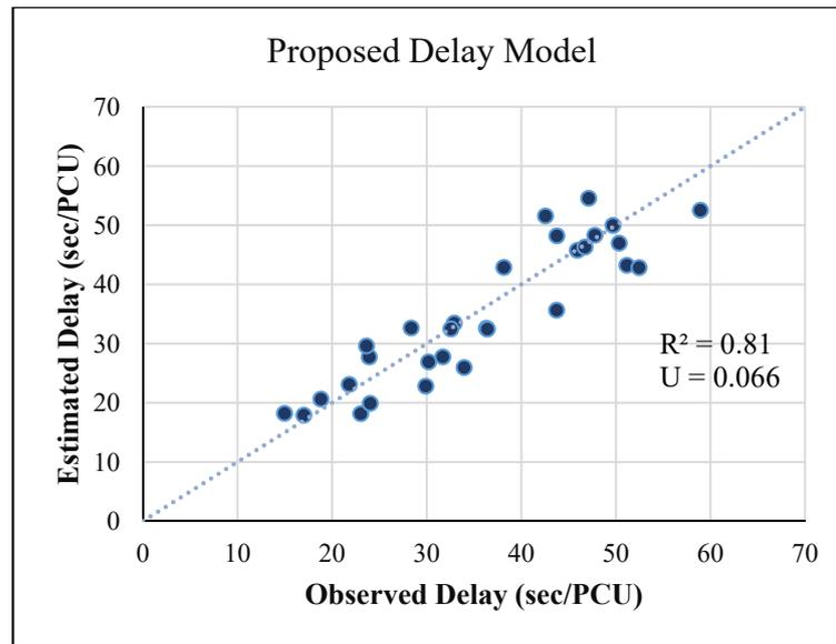
Figure 9: Correlation between the observed delay and the modified delay model estimate
