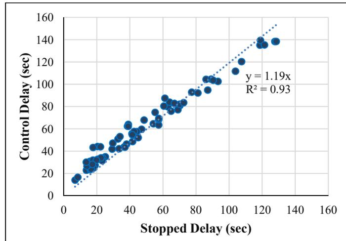
Figure 5: Relation between stopped delay and control delay
