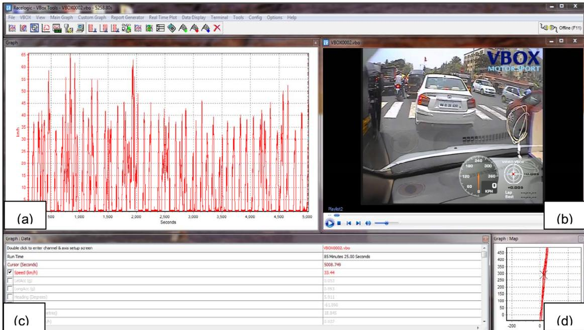
Figure 3: (a) Main window displaying speed against time (b) Video player window (c) The graph data (d) Graph map showing the path of vehicle.
