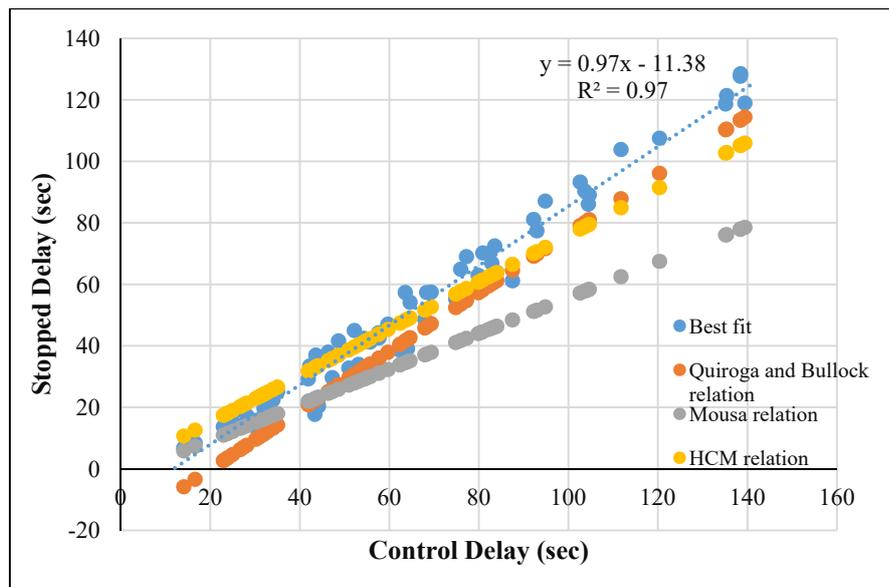
Figure 6: Comparison between stopped delay and control delay.
