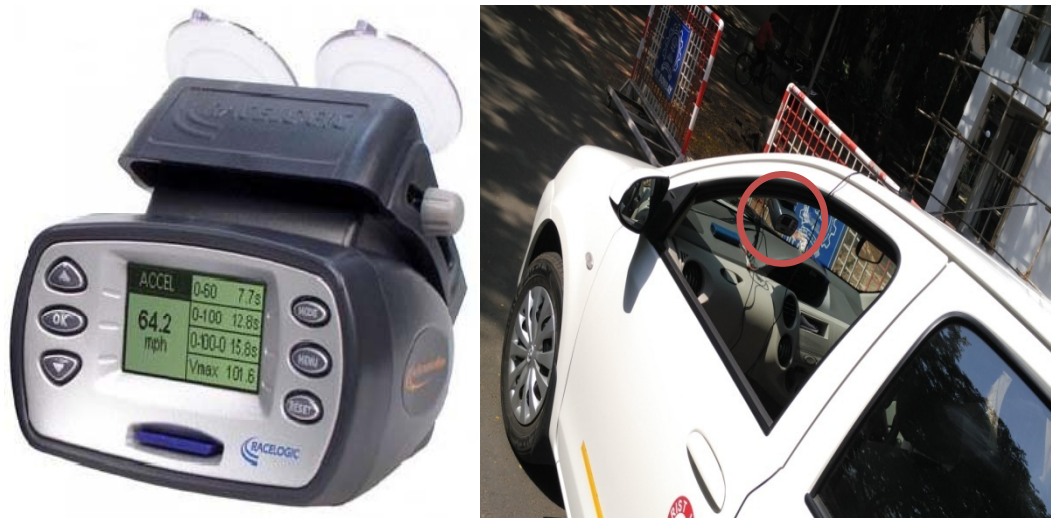
Figure 2: Showing Performance Box (Source: Racelogic Ltd, Performance Box Manual.) And performance box mounted in the test vehicle.
